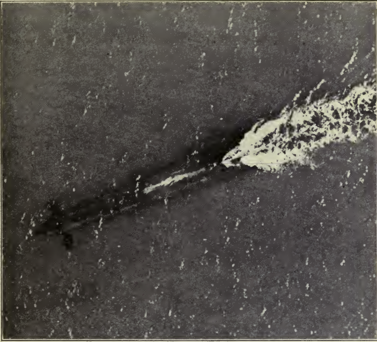
A submarine as seen from an aeroplane. The white foam of the submerged boat is caused by the conning tower which is not altogether under water.
